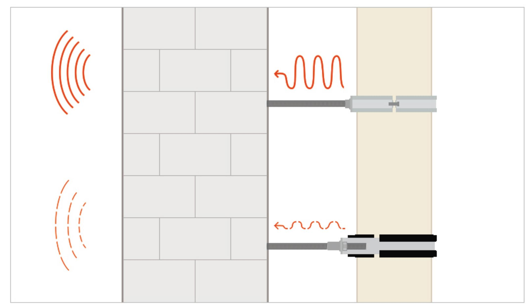
**Poliran RC** is specially designed for soundproof drainage systems and significantly reduces the structure-borne noise
